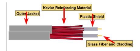
The light-guiding parts of an optical fiber are called the *core* and the *cladding*. The core is usually very pure glass with a high index of *refraction*.
